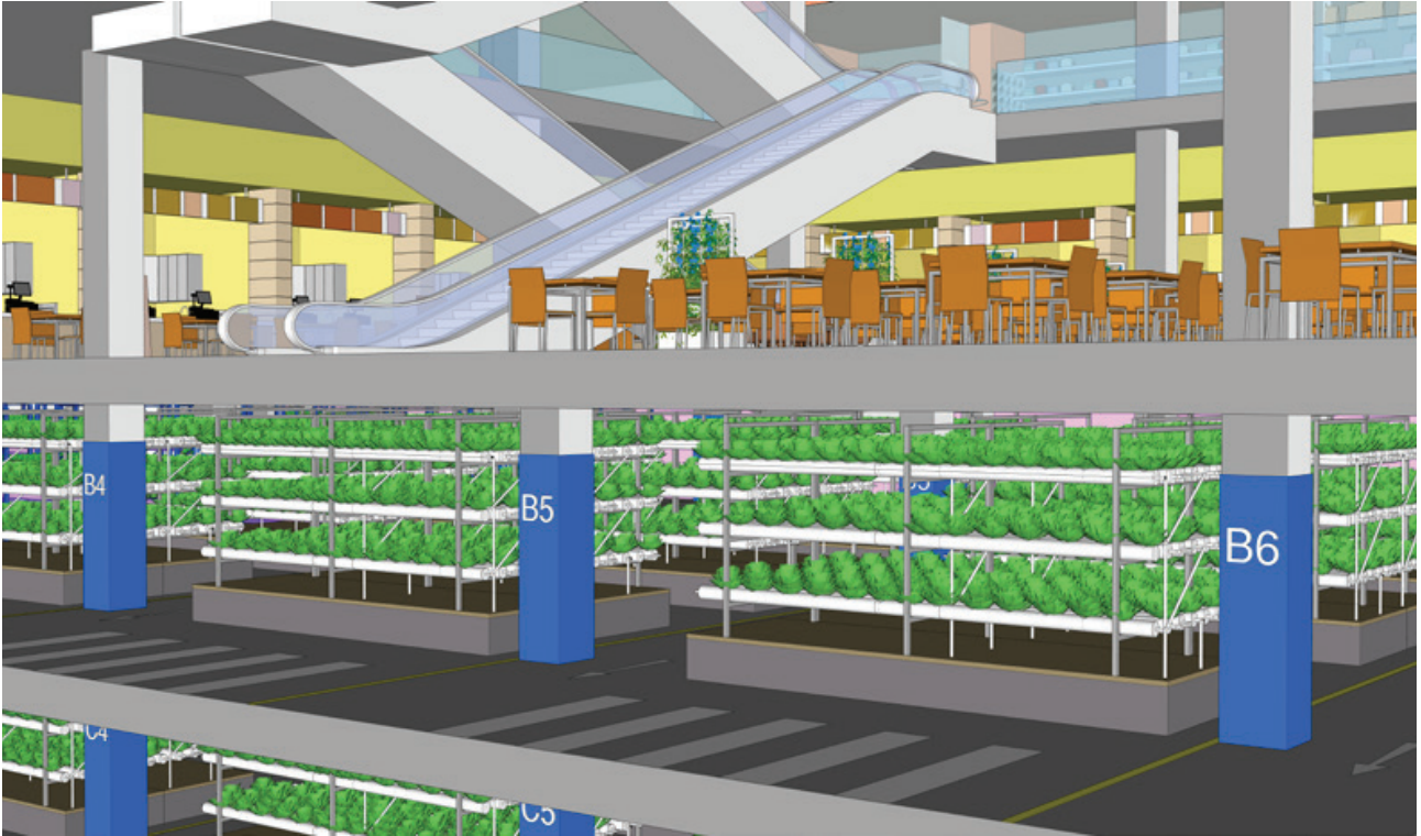
Fig. 7: Illustrative view of a retrofit department store, with public retail spaces above and vertical farming spaces below. © Arup
