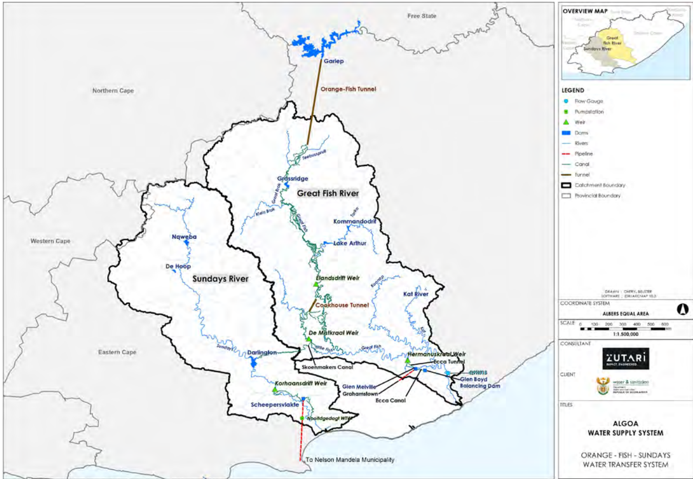
Figure 3-3. Overview of the Orange–Fish and Lower–Sundays River Transfer Scheme (DWS, 2022). The key supply and storage dams for NMBM are indicated in red.
