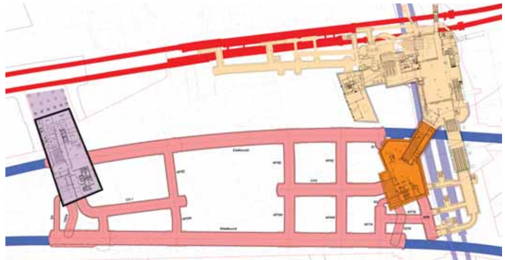
Crossrail contract C121 sprayed concrete-lined tunnels Goslett Yard box Existing LUL Central Line Crossrail contract C122 bored tunnels Crossrail Tottenham Court Road station LUL Tottenham Court Road station Existing LUL Northern Line
