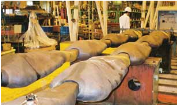
26. Cast steel elements connected.
