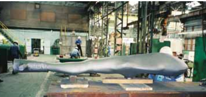
20. Cast steel piece before machine processing.
