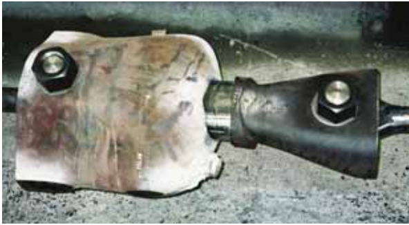
25. Shrink-fitted test piece for tensile strength testing.
