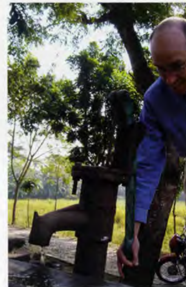
4. Pump from tube well.
