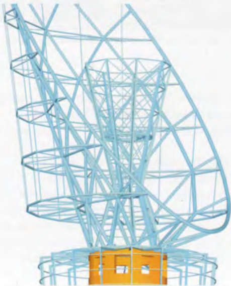
4. The flame cauldron and lattice shell structure.
