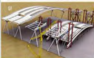
6. Roof assembly sequence.
