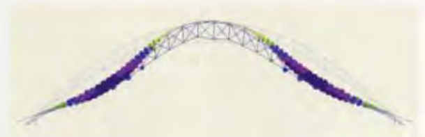
6. Lighting arch - push/pull buckling.
