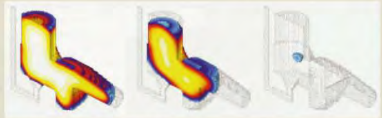
19. Computer modelling of casting solidification.
