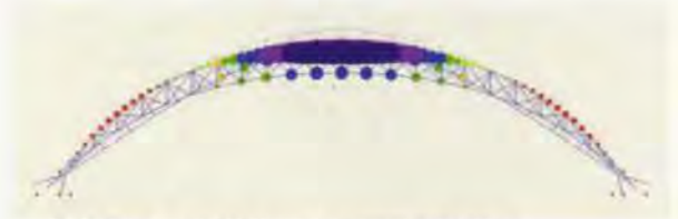
5. Lighting arch - Uniform compression buckling.
