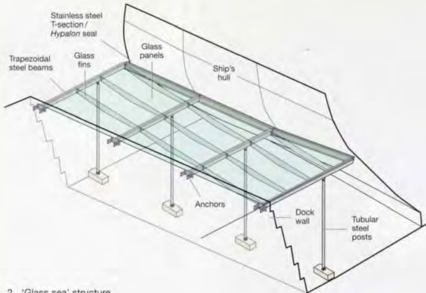
2. 'Glass sea' structure.
