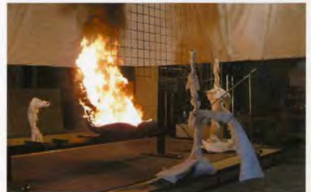
17. Combustion test on fire resistance of steel elements.
