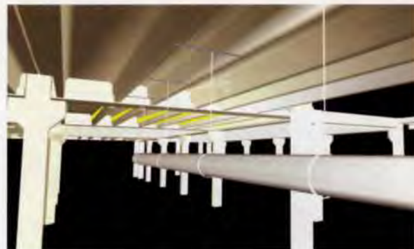
9. Services support system from precast 'T'.
