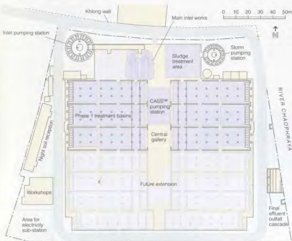
7. Plan of wastewater treatment plant.
