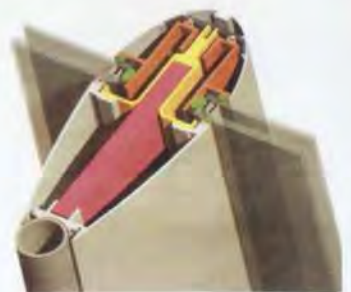
4. 3D rendering of aluminium glazing mullion.
