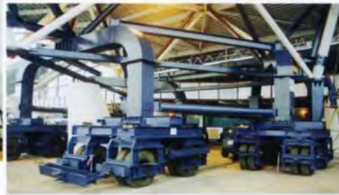
6. Blue-painted steel temporary carrying chassis beneath node.
