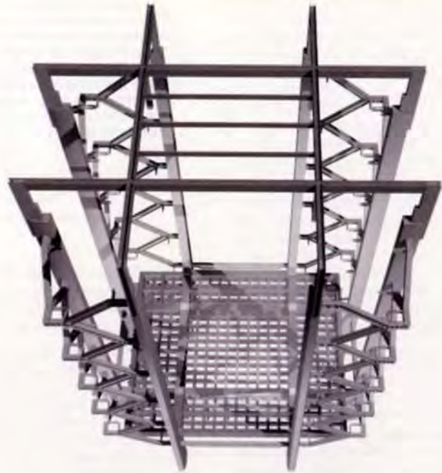
4. The dual seismic-resistant system: EBFs and MRFs.
