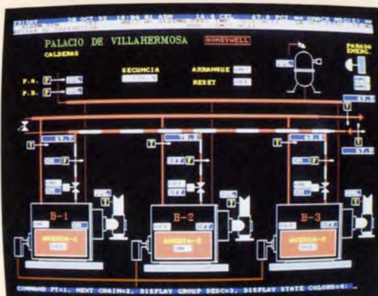
A. Building Management System panel display.
