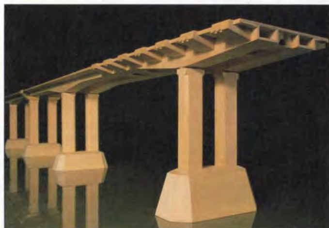
▲ 6. Model of precast post-tensioned concrete anchor span.
