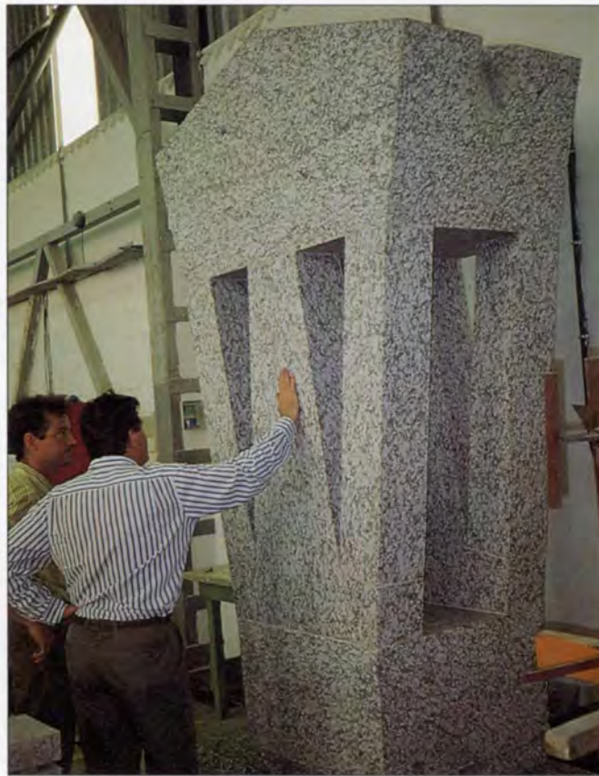
◀ 6. Peter Rice (back to camera) inspects prototype of stone unit for the Future Pavilion façade at the stonemason's workshop, July 1991. (Photo: Bruce Danziger)
