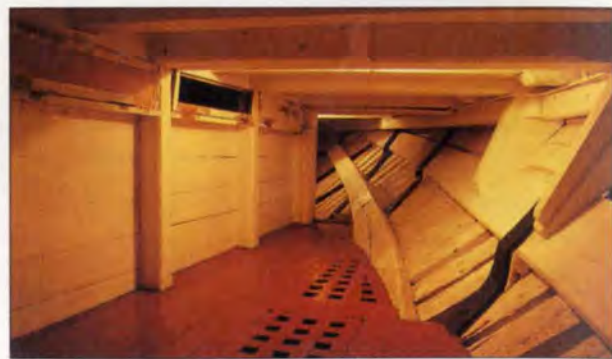
4. Some frame members were soaked in brine as an aid to preservation and marked 'SALT'.
