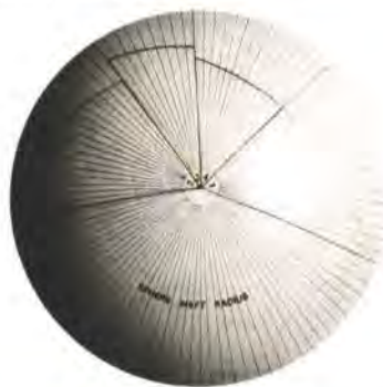
6. Sydney Opera House: model of segmented sphere solution to the design of the shells.
