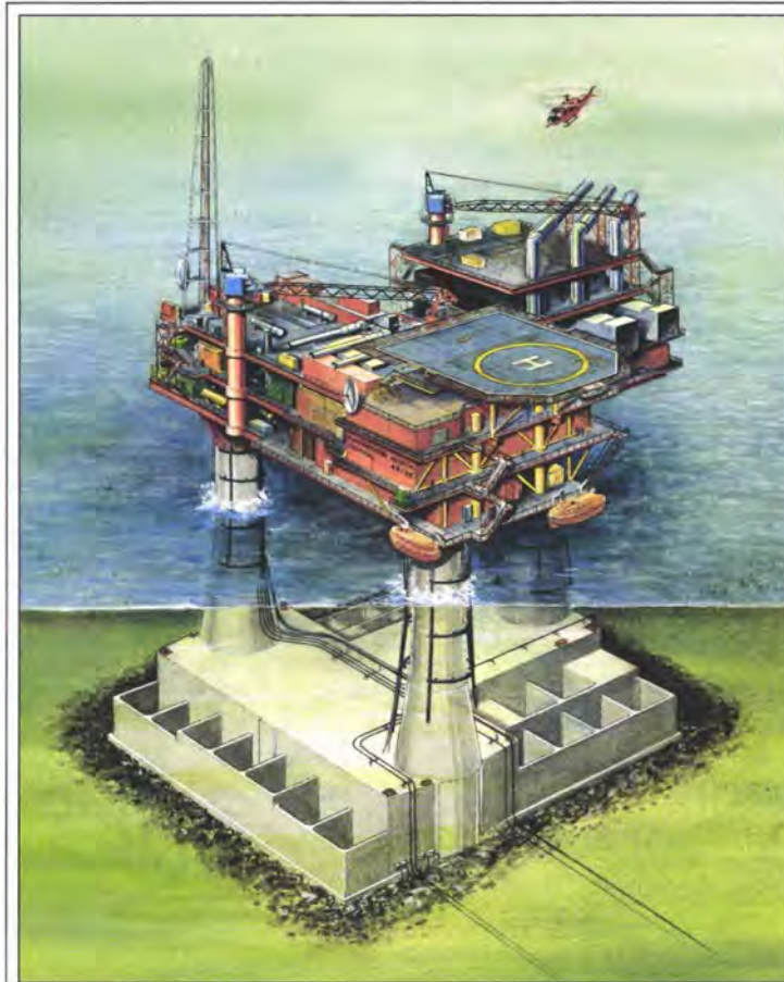
1. Impression of Ravenspurn North central processing platform after installation of both decks.
