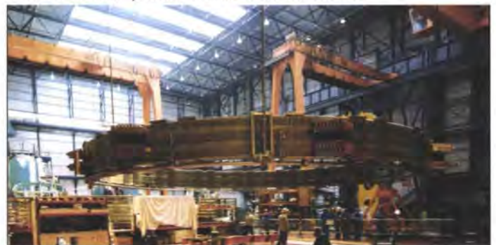
▽ 13. Lower outer poloidal field coil under construction
