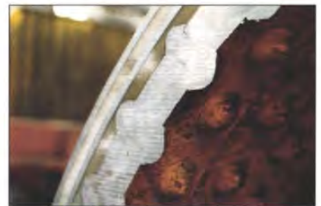
16. Band detail: Test piece sliced through after grout injection and tested to twice working pressure.
