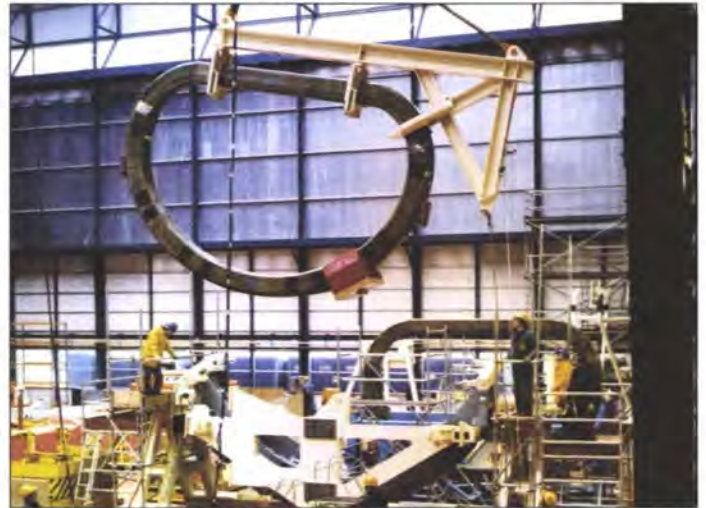
▽ 13. Lower outer poloidal field coil under construction
