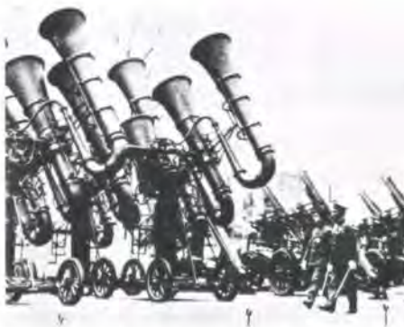
Fig. 14 Emperor Hirohito of Japan (left) with his chief of staff inspecting sound detectors for locating enemy aircraft, Osaka 1934
