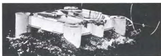
Fig. 2 Hutton TLP 1:33 model under maximum height, maximum steepness, regular waves in NMI main test tank, London
