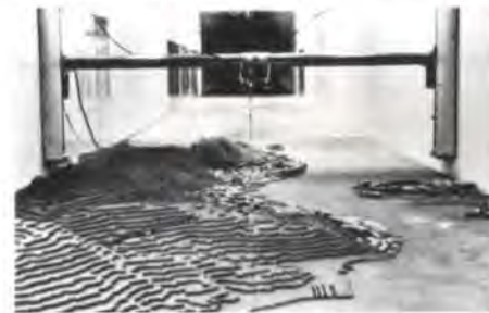
a) Layout of topographical model for wind tunnel tests b) Section of topographical model in wind tunnel c) 1:500 scale proximity model including proposed building
