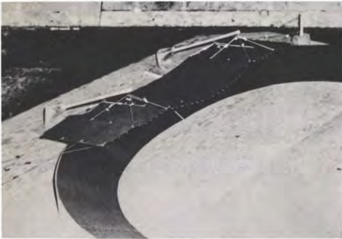
Fig. 3 Aeroelastic model for Berlin roof project, a heavyweight cable roof (Photo : Courtesy of Frei Otto)
