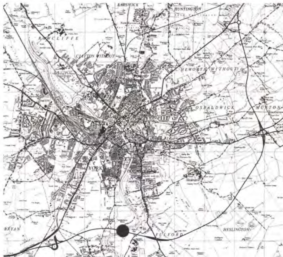
Fig. 1 The York Bypass will take through traffic on the A64 Leeds/Scarborough trunk road round the city of York. It will be a dual, two-lane road to near-motorway standard. 18 bridges have been built on the 14 km long road. We designed the River Ouse Bridge; the road and the other structures were designed by the Durham Sub-Unit of the North Eastern Road Construction Unit
