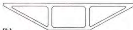
(b) Lighter in appearance but more expensive. The sloping slabs carry shear and therefore need to be prestressed but a single row of cables will have a high centre of gravity and therefore be inefficient
