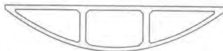
(c) The chosen cross section. Light in appearance. The cables in the shell can be draped between the top over supports and the bottom at mid span and therefore have maximum eccentricity at the critical sections
