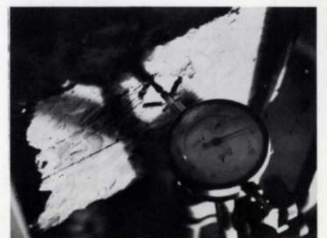
Fig. 8 End of test beam from diaphragm wall in test rig
