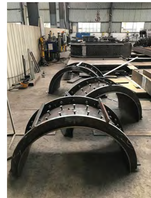
8. Arup designed steel arches to structurally enhance the historical brick archways
