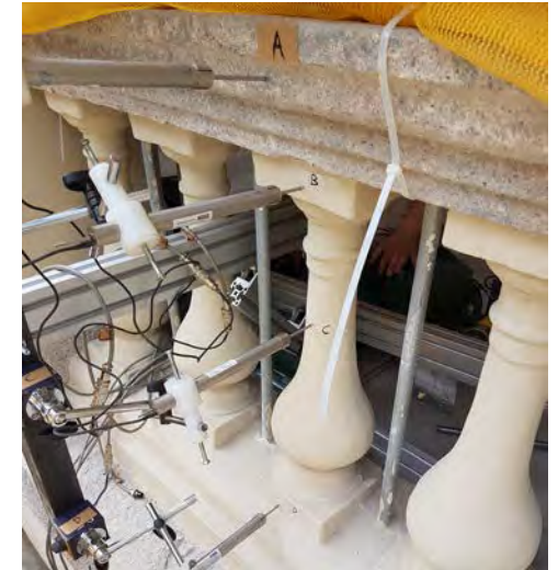
7. The reinforced balustrades were load tested to code requirements
